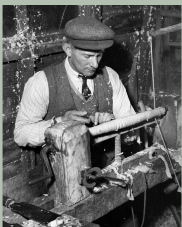
Alex Dean turning a chair leg on a pole lathe Andy Dean/Wycombe Museum
