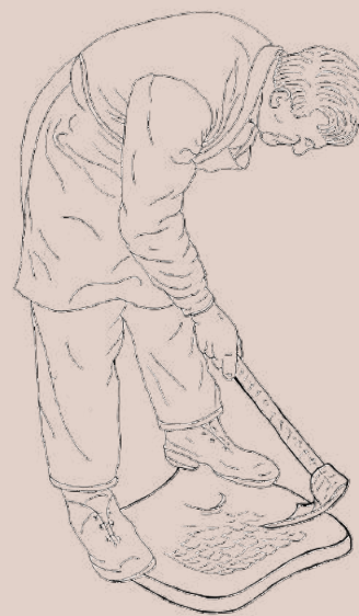
Bottomer adzing a chair seat Stuart King (from a photo in SWOP/Wycombe Museum)
