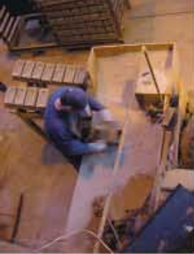
Brickmaking by hand using wooden moulds (Bovingdon Brickworks)
