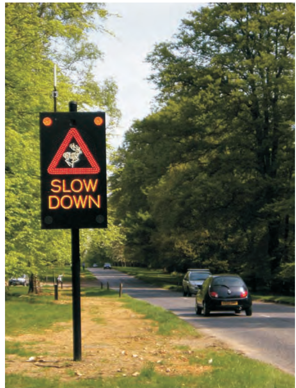
A dual-function VAS activated by animals crossing or vehicles exceeding a pre-set speed
