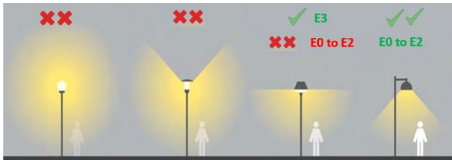
Fig 1: The correct luminaire distribution. [We need to redraw this image: only the far right configuration is appropriate within the Chilterns NL and its setting.]
